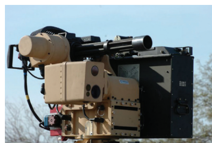
RWS fitted with Dillon Aero M134-Series minigun
